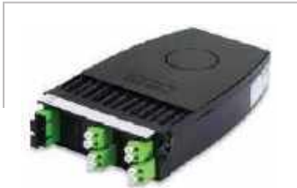
SCSU1208SLF, FX Ultra Splitter Cassette, OS2, Single 2x8 Splitter, SC/APC Upstream Ports, LC/APC Downstream Ports
